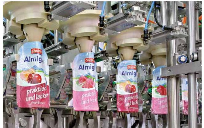
Besides precise filling and high speed the sterility and storage life are the major challenges when filling fresh, liquid dairy products into pouches. This is where SN's concept is convincing. On meanwhile three SN Ultra Clean FFS machines of the LMS series achieved Ehrmann today has a product shelf life of 60 days.
